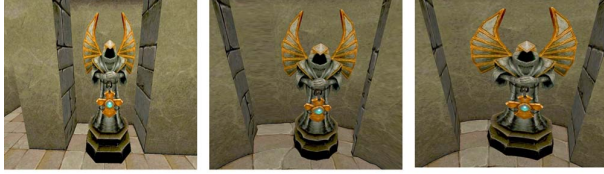
Figure 4: Conventional rendering for ground truth (left), rendering using our method with both the global and local detail-preserving steps (middle), and rendering using our method with only the global step (right). The local step alleviates the stretching of the statue.
